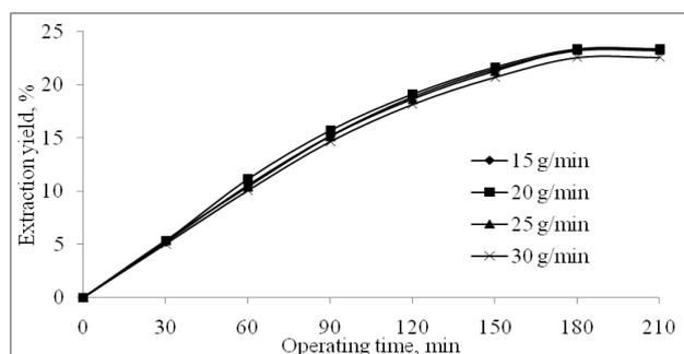
**Figure 4- Effect of supercritical carbon dioxide flow rate and operating time on extraction yield**
