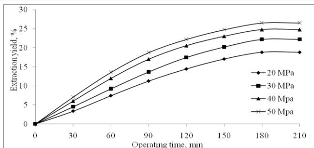
**Figure 2 -Effect of extraction pressure and operating time on extraction yield**
