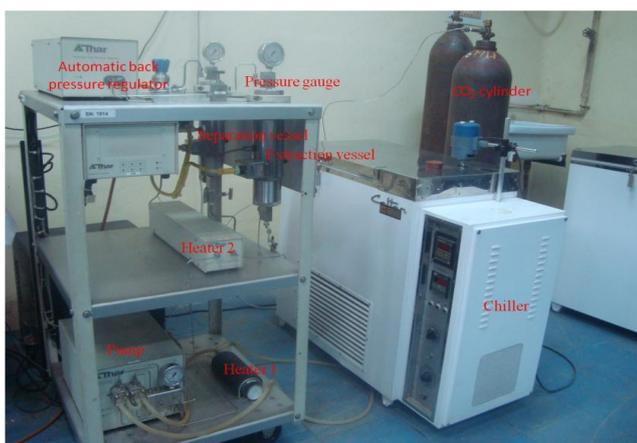
**Figure 1-Semi – continuous supercritical carbon dioxide extraction unit**
