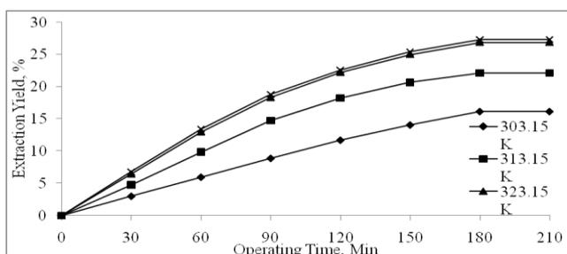
**Figure 3-Effect of extraction temperature and operating time on extraction yield**
