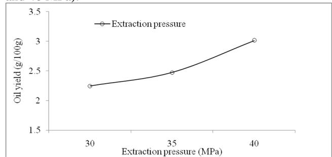
**Figure 1- Effect of extraction pressure on extraction yield**
