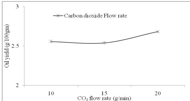
**Figure 3** Effect of volumetric CO<sub>2</sub> flow rate on extraction yield
