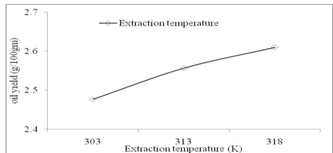
**Figure 2 - Effect of extraction temperature on extraction yield**
