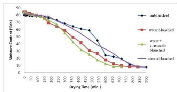
**Figure 2: Changes in Moisture Content with Time During Drying of Untreated and Pre Treated Fenugreek Leaves at 50 °C**
