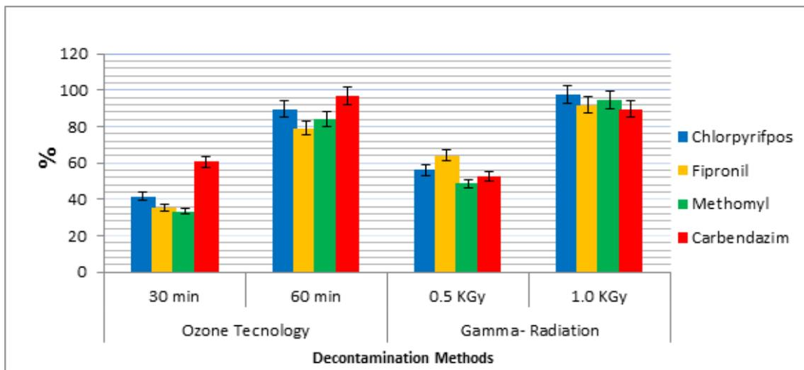
**Figure 2: The Efficiency of Decontamination Techniques for Reduction of Pesticides Residues in Date Palm Fruits in Comparison with the Initial Level**
