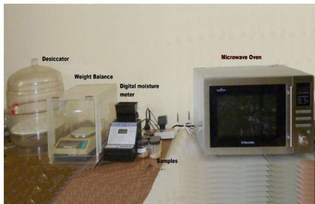
**Figure 1** Pictorial view of Whole moisture analysis system (including standard moisture meter and microwave oven based technique)
