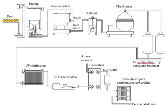
**Fig.1 Schematic representation of process for concentration of fruit juices**
