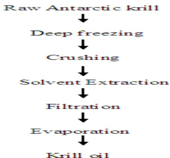
Figure 4: Krill oil extraction process
