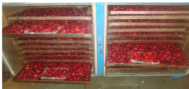
Figure 1- Drying of kokum rind in the tray dryer and weight was recorded by using small perforated trays
