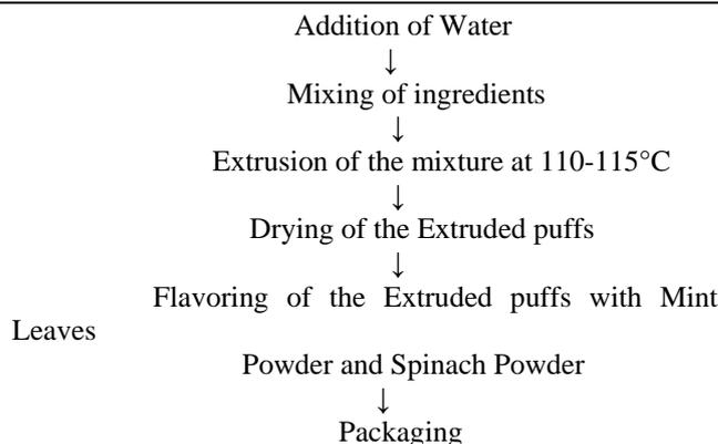
**Fig 1 Flowchart for the Development of Extruded Fortified Corn Snack for different treatments**
